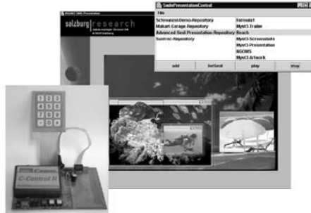
Fig. 2. The SMIL player (middle) being controlled either by a micro-controller (left) or by the control GUI (right)
